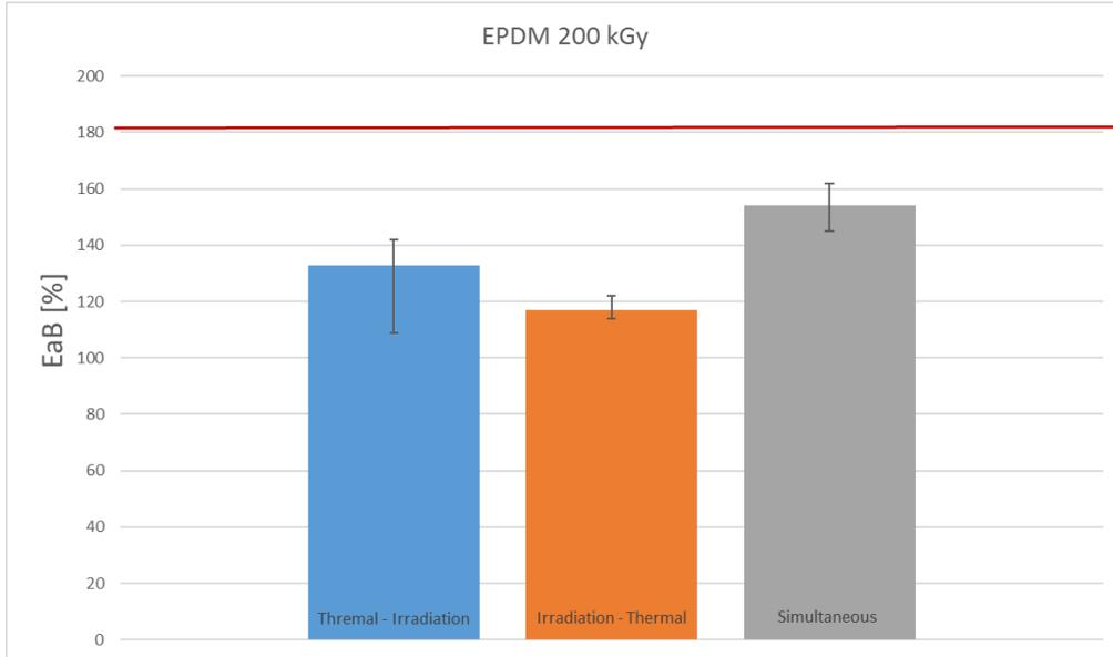
Figure 6. Comparison of sequence of ageing on EPDM samples. Blue column describes the decrease in EaB when sequence is thermal-irradiation, orange column irradiation-thermal and grey column simultaneous thermal and irradiation ageing.
