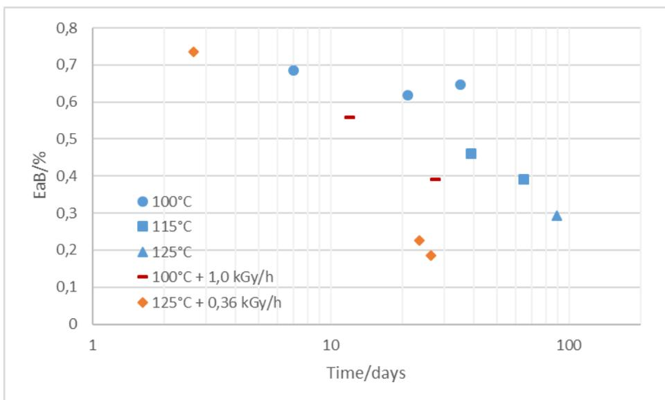
Figure 14. Ageing data from the combined thermal and irradiation environment (red and orange markers) and the formed master curve at 100°C from thermal only ageing data (blue markers).
