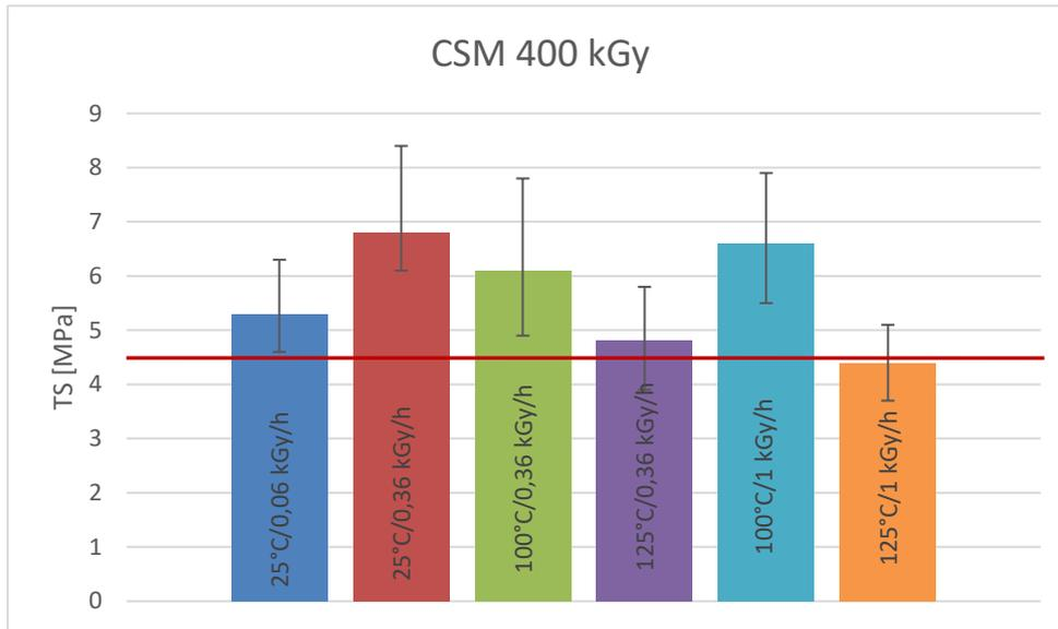
Figure 10. Tensile stress (TS) results for CSM samples irradiated with calculated dose of 400 kGy. The red horizontal line presents the non-aged material TS value of 4,5 MPa.
