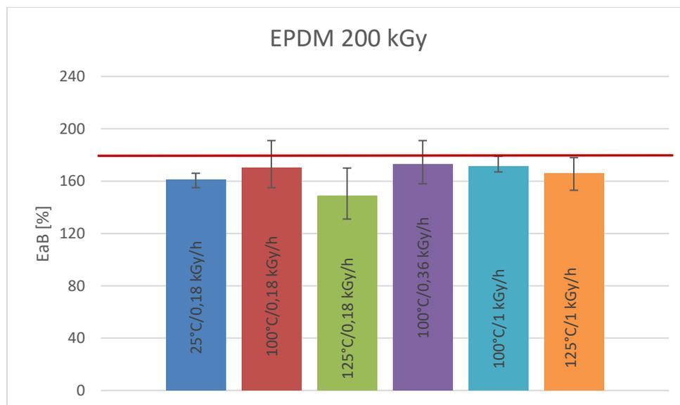
Figure 2. EaB results for EPDM samples irradiated with calculated dose of 200 kGy. The red horizontal line presents the non-aged material EaB value of 182%.
