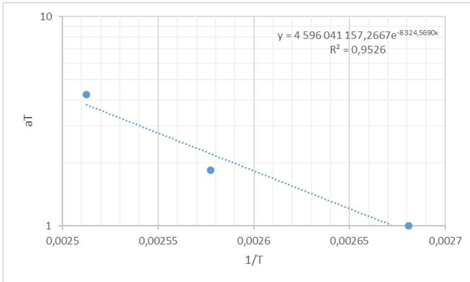
Figure 13. Extracted shift factor values versus 1/T.
