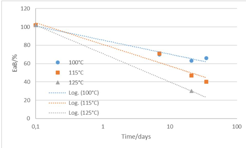
Figure 11. Evolution of EaB at three different temperatures as a function of exposure time.
