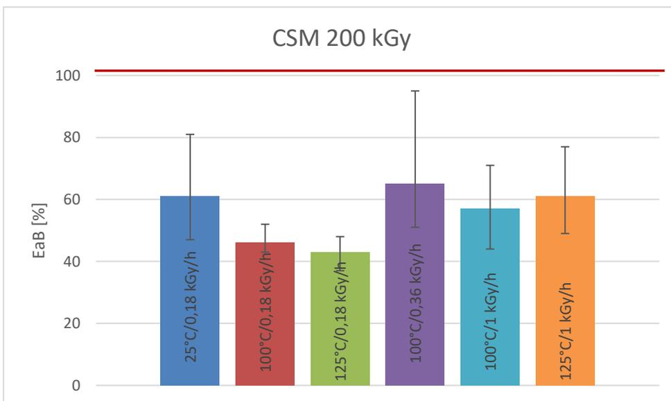
Figure 7. EaB results for CSM samples irradiated with calculated dose of 200 kGy. The red horizontal line presents the non-aged material EaB value of 102%.
