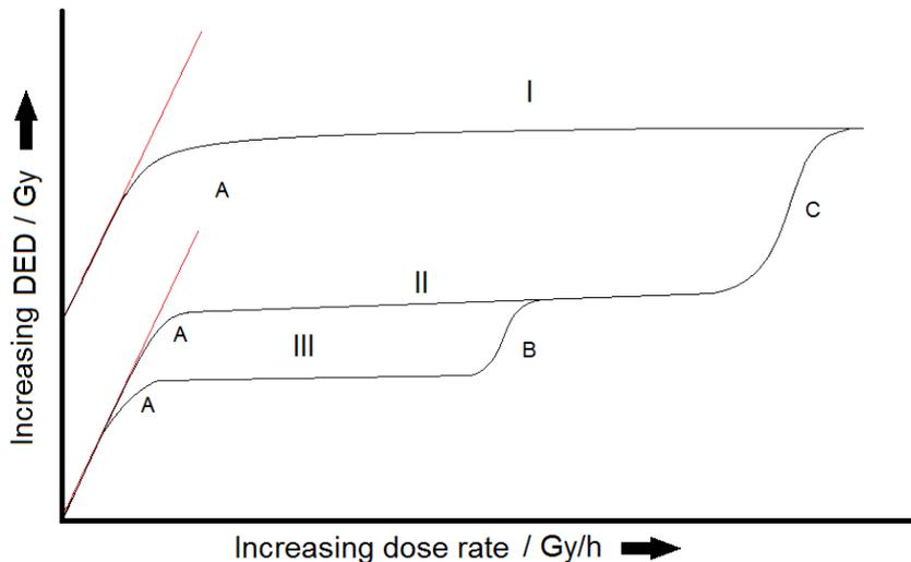
Figure 1. Schematic illustration of the dose rate effect.
