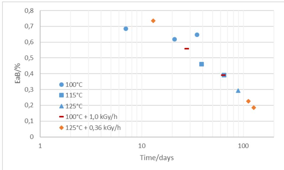
Figure 15. Master curve at 100°C combining thermal and thermal-radiative data.
