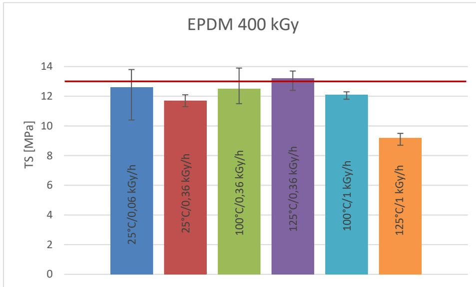
Figure 5. Tensile stress (TS) results for EPDM samples irradiated with calculated dose of 400 kGy. The red horizontal line presents the non-aged material TS value of 13,0 MPa.
