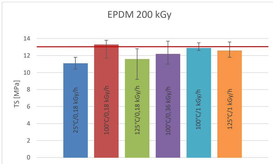
Figure 4. Tensile stress (TS) results for EPDM samples irradiated with calculated dose of 200 kGy. The red horizontal line presents the non-aged material TS value of 13,0 MPa.
