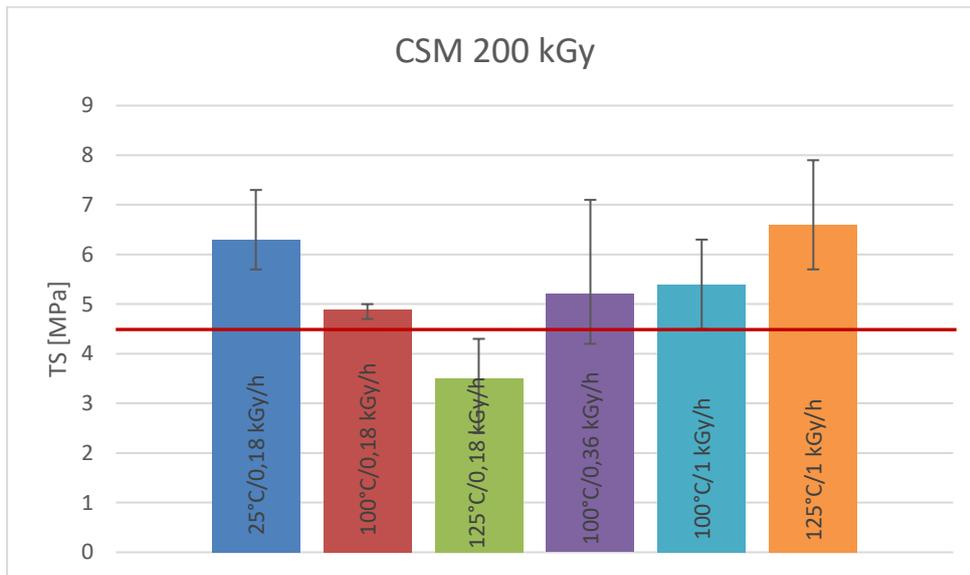
Figure 9. Tensile stress (TS) results for CSM samples irradiated with calculated dose of 200 kGy. The red horizontal line presents the non-aged material TS value of 4,5 MPa.
