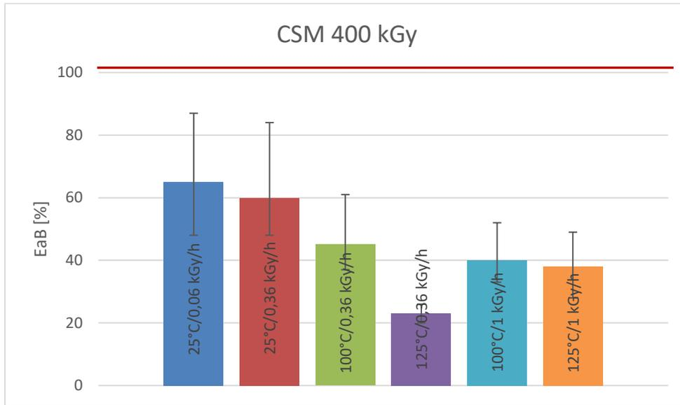
Figure 8. EaB results for CSM samples irradiated with calculated dose of 400 kGy. The red horizontal line presents the non-aged material EaB value of 102%.
