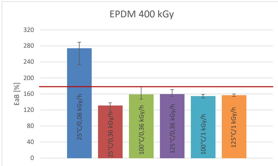
Figure 3. EaB results for EPDM samples irradiated with calculated dose of 400 kGy. The red horizontal line presents the non-aged material EaB value of 182%.
