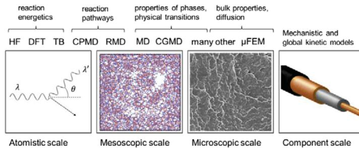
**Figure 6.** Scales and processes of thermal and radiation ageing coupled with numerical modelling methods.
