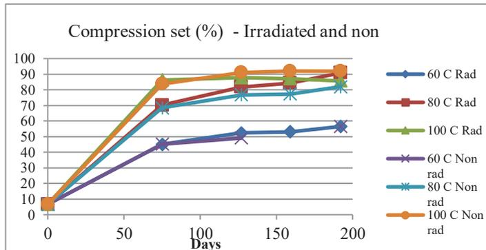
**Figure 4.** Compression Set for Nitrile Rubber.
