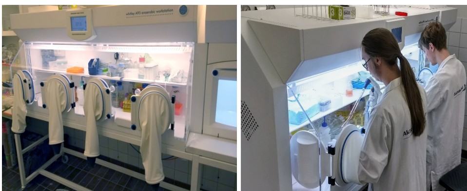
Figure 2. The workstation uses a special gas mix to maintain a highly anaerobic environment and is able to support two users.
